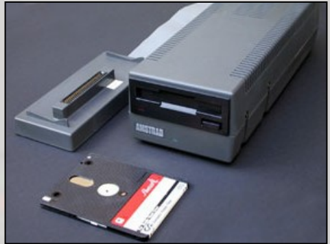
AMSTRAD FD-1, 3 INCH DISK DRIVE WITH A DDI-1 INTERFACE CONTAINING THE AMSDOS ROM
