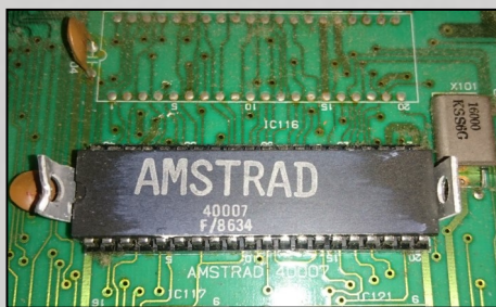
BENEATH THE HEATSINK, THE AMSTRAD 40007
